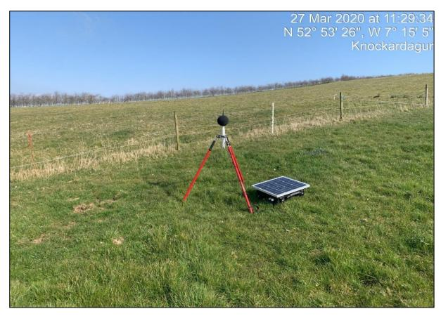
Figure 11.2: Noise Measurement Equipment
